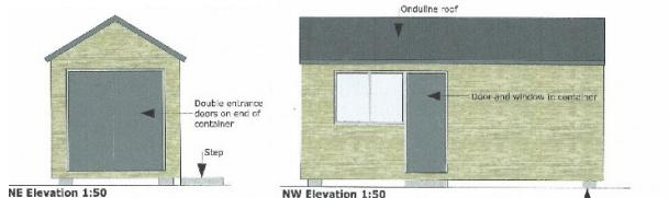
The facility (above) will be approximately 20ft long x 8ft wide x 8ft 6in high (11ft 6in to the roof ridge). It will be clad in a material suitable to its location and have a low pitched, black, organic fibre roof to blend into its rural environment.
